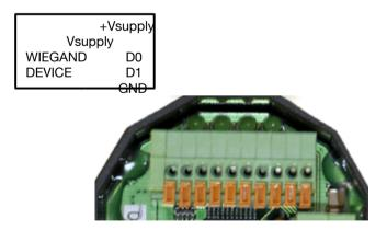
The WIEGAND interface is enabled by setting Bit 6 of register 274 (Reg. 274 OR 40h).
