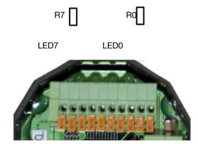
**TTL devices on I/O** Each BARIX X8 I/O can be set to work either as input or output. External device TTL level I/Os can be attached to the I/Os and to signal ground as shown in the schematic below.
