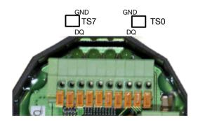
At Power-Up the BARIX X8 is scanning all 8 inputs (I/O0 - I/O7) for attached TS sensors. Each found sensor is represented by the corresponding Bit in the High Byte of register 11:
